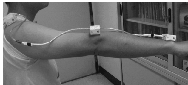
Fig. 1 Illustration of three inertial sensors mounted on the upper limb, conducting a triangle movement
